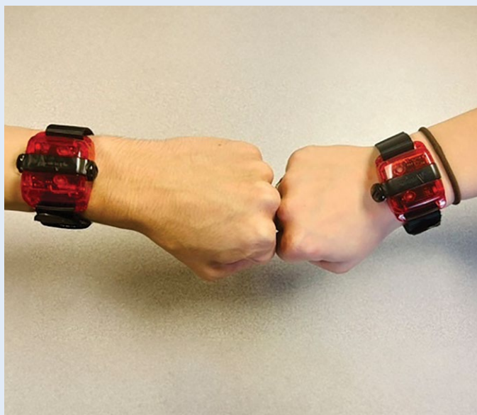
Undergraduate research assistants show off the actigraph, a device designed to measure sleep-wake cycles.
